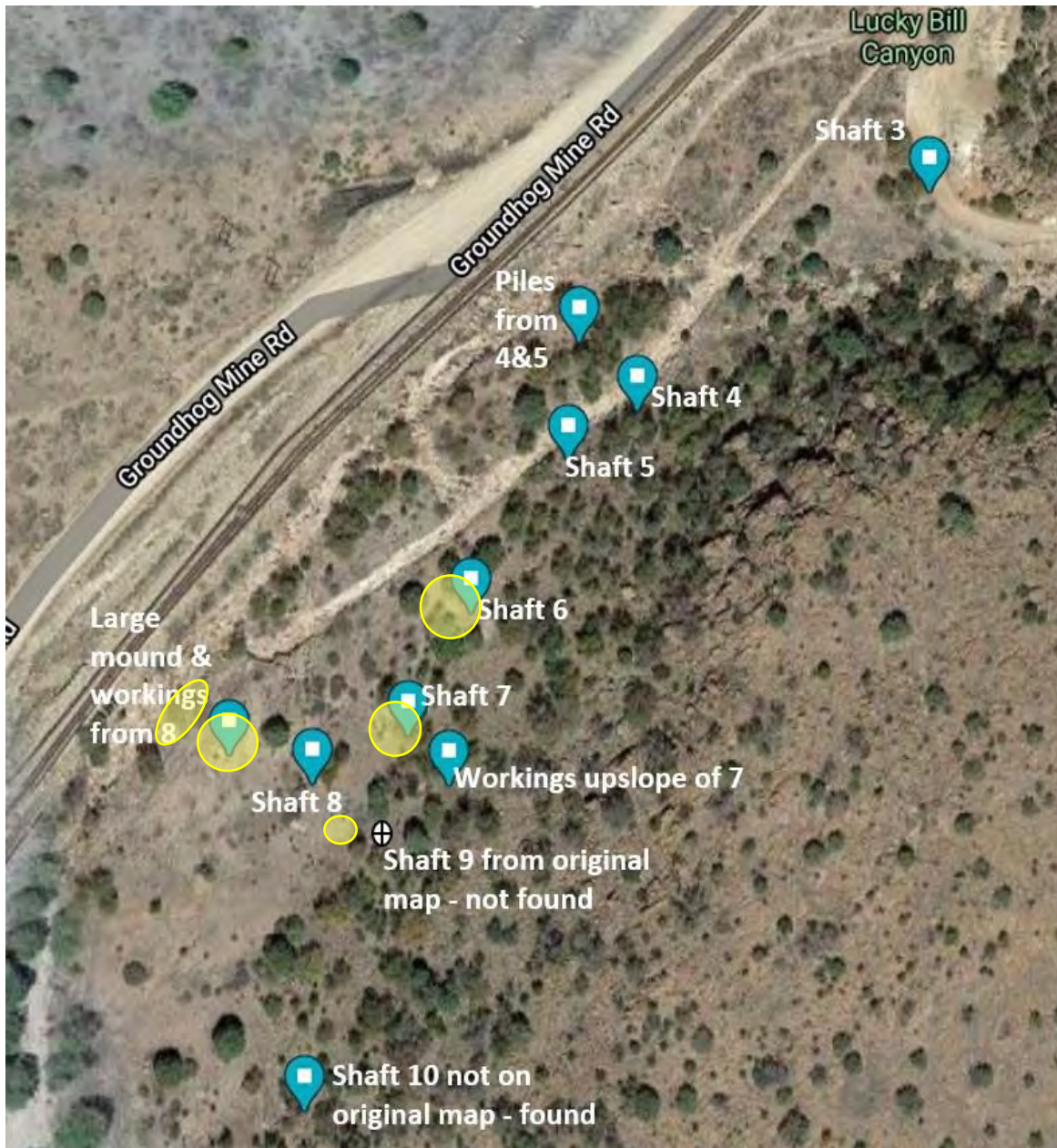
Figure 1: Central portion of site. Shared Services excavated 3 small areas identified by NMED along creek bank (oval) plus additional material encountered beneath bank surface. Finished removing material around Shaft 7, and a small reddish area SE of Shaft 8. Removed entire mound and area beneath it. Started removing material at Shaft 6.
