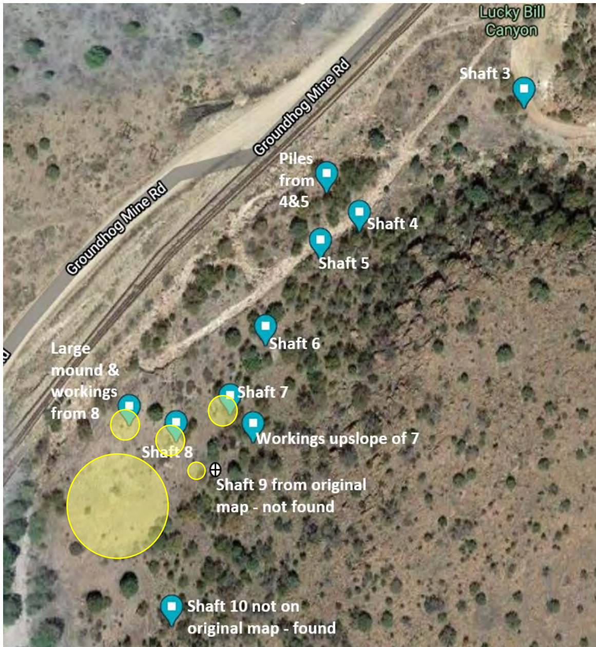
Figure 1: Central portion of site. Shared Services expanded boundaries and depth of primary excavation within large circle. Crew also removed soil associated with Shaft 7, Shaft 8, a large earthen mound, and a small reddish area east of Shaft 8.
