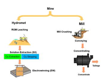
Figure 14.1 – Site Process Diagram
