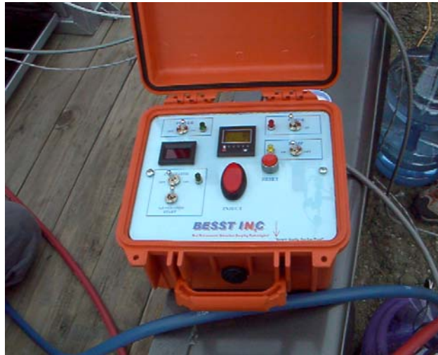
Figure 4: Dye Injection Control Unit for to-the-second regulation of dye injection pulses.
