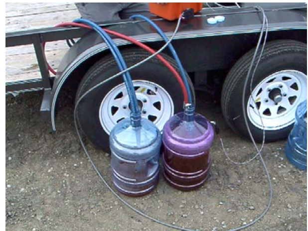
Figure 6: Bottle to right contains primary RR reservoir. When the large oval red button is depressed on the Dye Injection Control Unit (Figure 4), the RR solution is fed from the red tube, then to the injection pump, and finally through the injection nozzle and into the well. When the injection pump is idling, the RR solution circulates through the blue tube and red tube in the primary RR reservoir bottle. The secondary RR bottle receives excess RR that is not used during an injection pulse.
