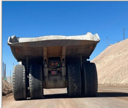
Passing green light installed on haul truck and rubber tire dozer.
